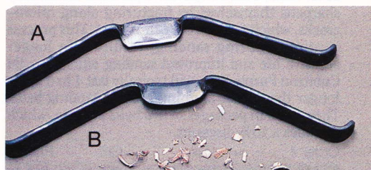
B. Finishing Hatchet has a thinner blade and is designed for finish and detail cuts. Its weight is 28ozs, blade width is 3¾" and overall length is 16".
