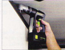
Right Angle Chuck drills in tight spaces
